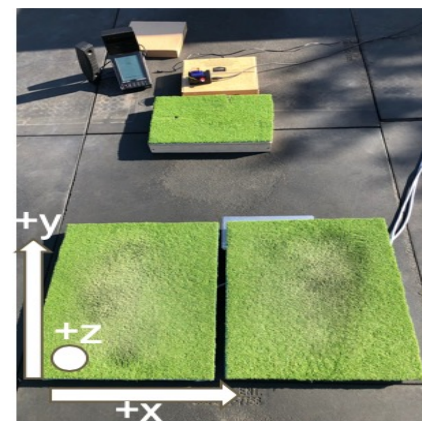
Figure 2: Showing turf on top of two force plates and the reference system utilized
